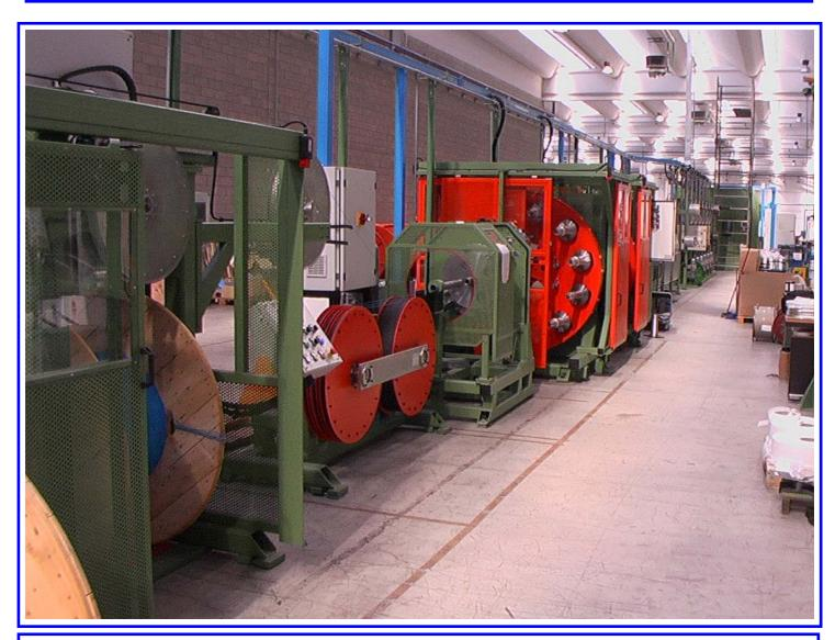
Line for laying up of cables composed by optical fibres in loose tubes or tight coated fibres. The equipment also allows the possibility of laying up also in double crown up to 19 elements.
